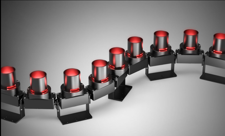
3D LED Flex 40 IP66 system. Each module comprises 4 x Luxeon Z red LEDs with a Gaggione ultra-narrow beam lens, and custom height anti-glare snoot. Each module is individually addressable via DMX
